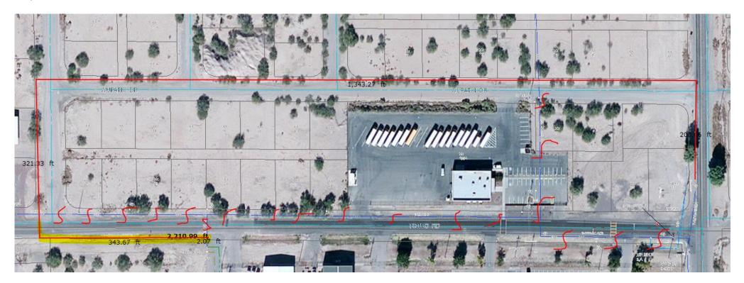
Red line = overhead line Yellow highlight = underground line S = removal of old overhead lines
