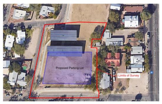
Full topo/culture survey for limits of survey boundary. Need 0.5-foot contours. Pick up bottom and top of wall shots at all wall locations. Pick up any visible utilities and/or bluestake marks.
