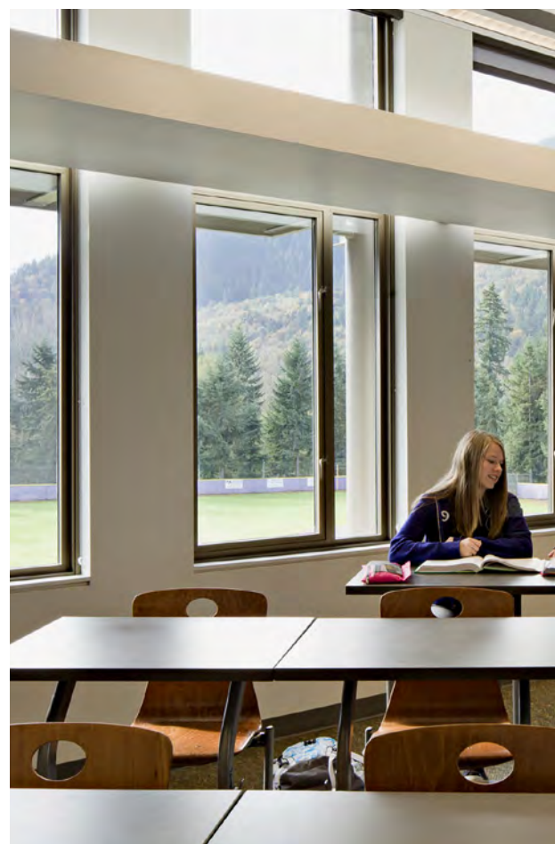
Classrooms incorporate windows, a light shelf to bounce light, direct/indirect pendant light fixtures and allow for views to a distant landscape. (Issaquah High School, Issaquah, WA; Mahlum)
