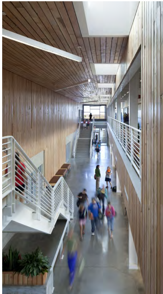
Sealed concrete floors requiring no finish, no toxic cleaning materials, and no finish replacement over time are incorporated in both the classroom and public spaces. (Kiowa County Schools, Greensburg, KS; BNIM Architects)
